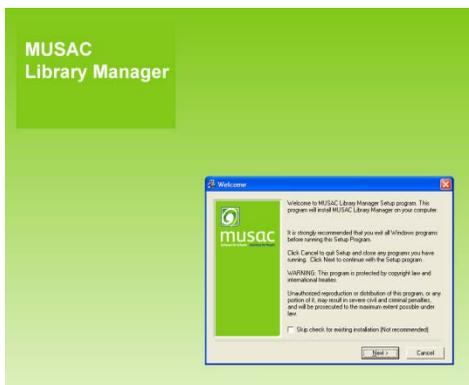
The program setup itself only needs to be installed once (on your network drive). Note that shortcuts will need to be manually added to other workstations.
